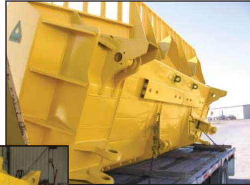
D11R HD Abrasion U Blade 21' wide, 45yd capacity
