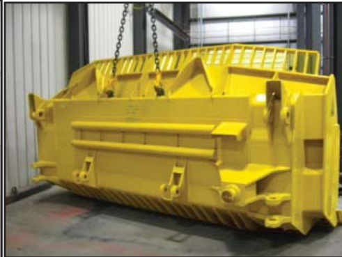
D10R/T HD Abrasion U Blade 17' wide, 28.8yd capacity
